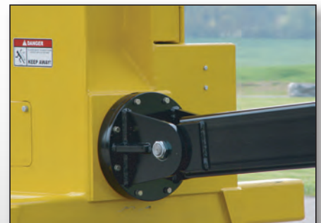
Heavy-duty bearing on each end of the swing-arm.
